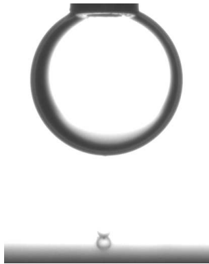
Figure 2.6: The detachment process leads to the deposition of a tiny drop on the surface, likely as a result of the dynamic of the instability process.
